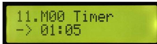
Push ▲ / ▼ to select the desired time CNC machine stops periodically.
