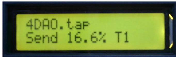
LCD screen have 16x2 characters, display the file list, sending/receiving status, setting parameters, errors alert, etc.
