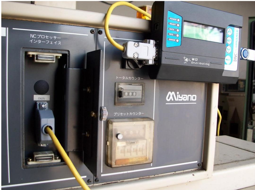
Installation of the machine with RS232 connection, external powered adapter:
