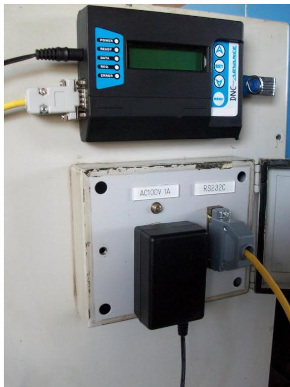
**!** Need to turn off the power of CNC machines before installing DNC One, or before removal DNC One. The installation online can cause problems for RS232 connection.
